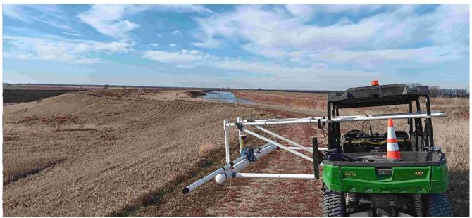
Gator UTV with EM geophysical unit parked on a levee
